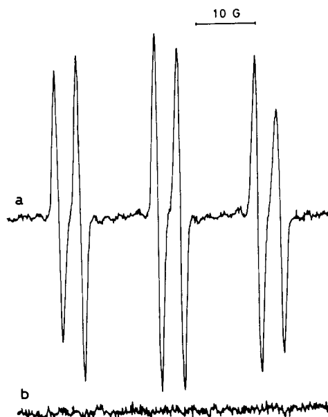
Fig. 2. The ESR spectrum of the BPN-hydroxyl radical spin-adduct obtained by carbazilquinone and NADPH-cytochrome P-450 reductase in the presence of BPN: (a) complete system, and (b) complete system + catalase. The signal was recorded after 15 min in (a) and 10 min in (b).
